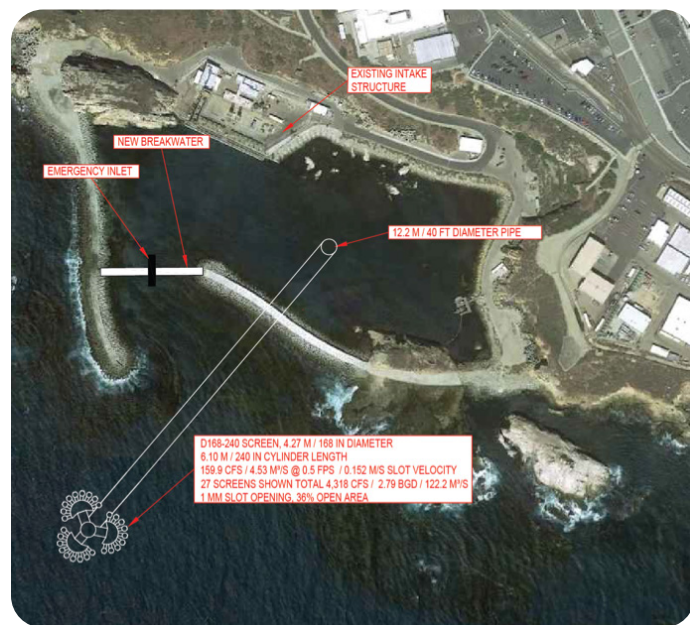
Figure 2. Aerial view of DCNPP with extended breakwater to isolate lagoon, emergency inlet structure, tunnel extending offshore, and wedgewire screen array for Option 1 configuration outlined in Figure 1.
