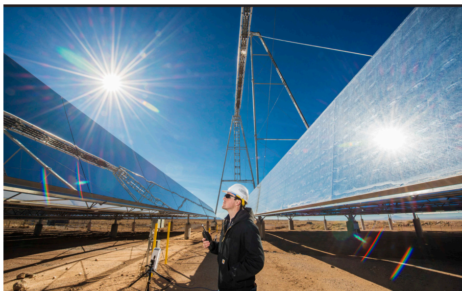
The molten salt test loop (MSTL) at Sandia National Laboratories' National Solar Thermal Test Facility in Albuquerque, New Mexico. The mirrors, based on AREVA's Compact Linear Fresnel Reflectors, focus sunlight to the top of the structure where molten salt is flowing. The resulting heat is stored and used later when the sun is not shining. Source: US Department of Energy
