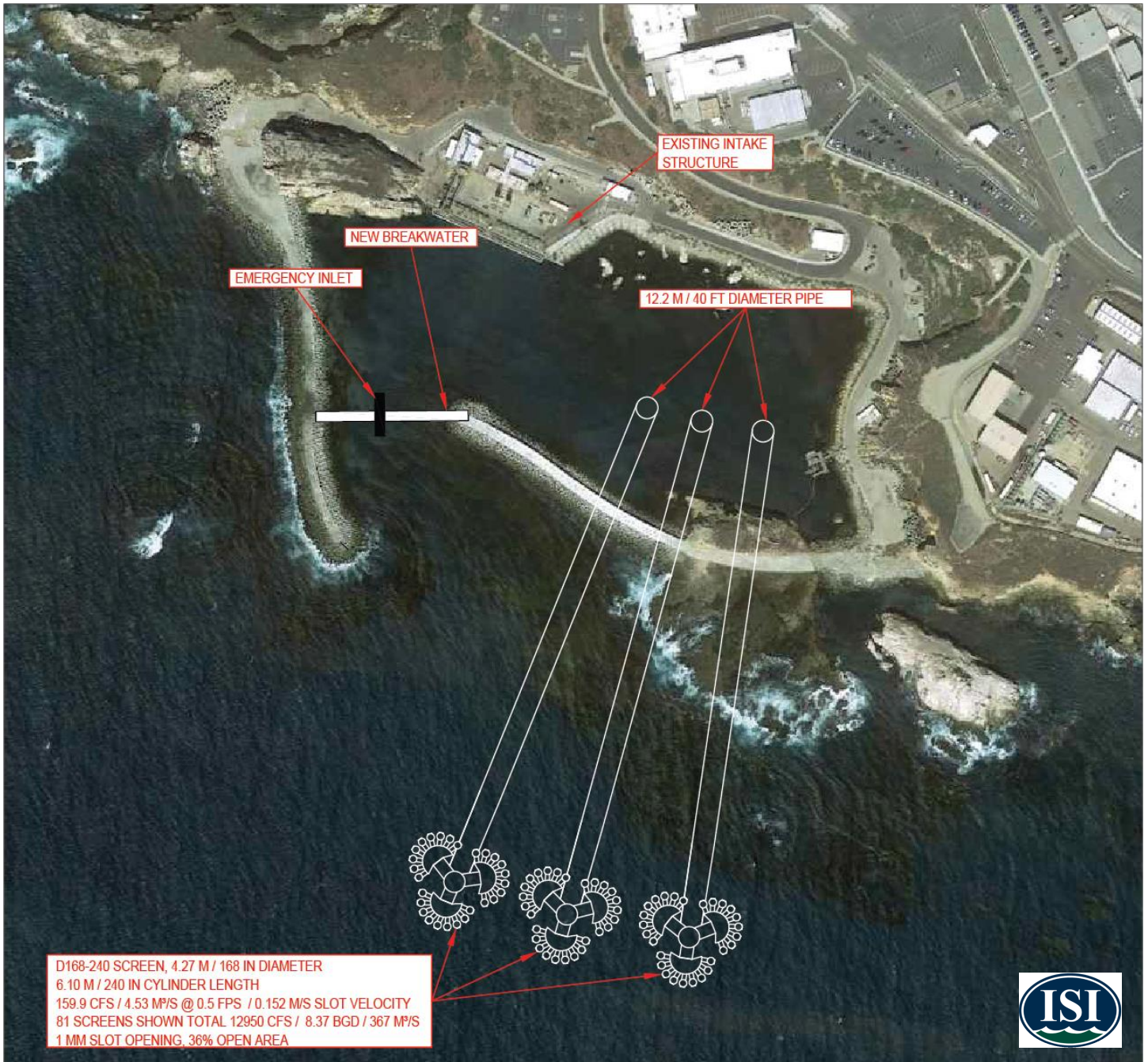
Figure 8. Aerial View of Diablo Nuclear Power Plant with Breakwater Extended to Isolate Lagoon, Emergency Inlet Structure, Tunnels Extending Offshore and Wedgewire Screen Arrays for 356 m 3 /s Option
