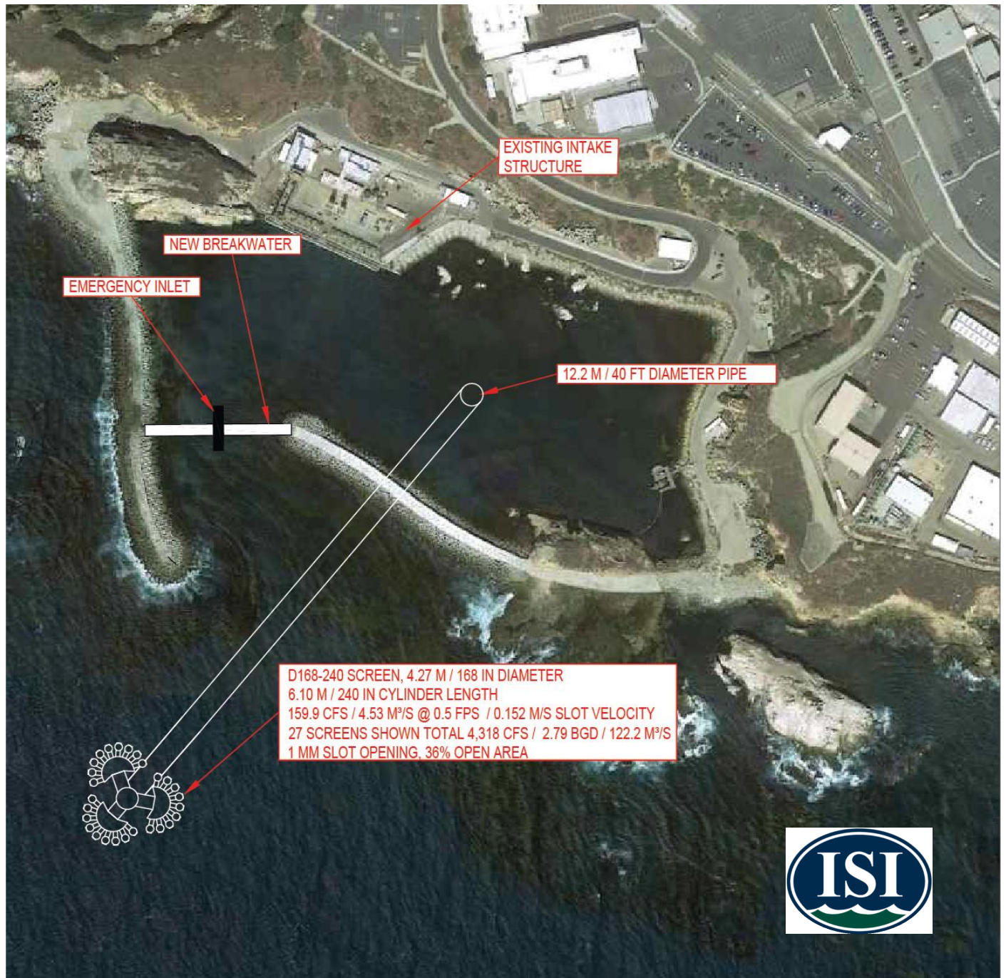
Figure 6. Aerial View of Diablo Nuclear Power Plant with Breakwater Extended to Isolate Lagoon, Emergency Inlet Structure, Tunnel Extending Offshore and Wedgewire Screen Array for 110 m 3 /s Option
